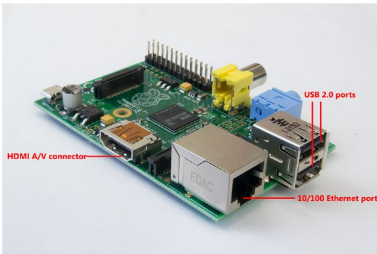
Figure 1-5. Raspberry Pi Model B's HDMI port, Ethernet port, and dual USB 2.0 ports
