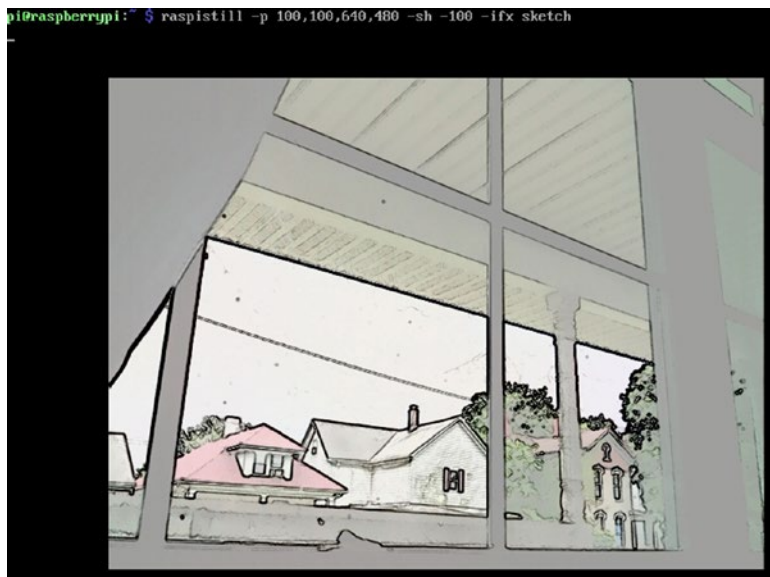
Figure 7-9. A demonstration of the -ifx sketch special effects setting with raspistill
