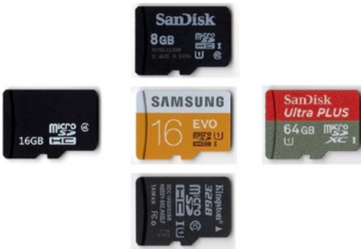
Figure 3-2. 8GB, 16GB, and 32GB microSD cards can be used by Raspberry Pi without reformatting. However, a 64GB card must be reformatted as FAT32 before it can be recognized.
